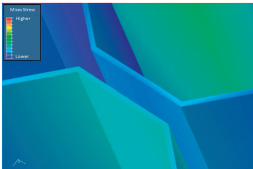
Figure 8. Unbonded node analysis close-up view showing tendency to separate.
